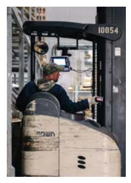
Thor VM1A Vehicle-mounted Computer, Granit Rugged Handheld Scanner
