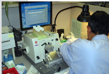
microtome station: barcoded cassettes are scanned to print barcode slide labels on demand
