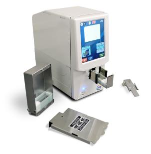
The SlideTrack ESPO slide printer provides an on-demand solution to printing text and barcodes on slides anywhere in your lab – including at the microtomy station. It features 300dpi thermal transfer printing technology to print text and barcodes directly on the slide surface. Two magazines hold 100 slides each for continuous printing, while the front loading feature enables single slide printing for control sides with tissue on the slide.
